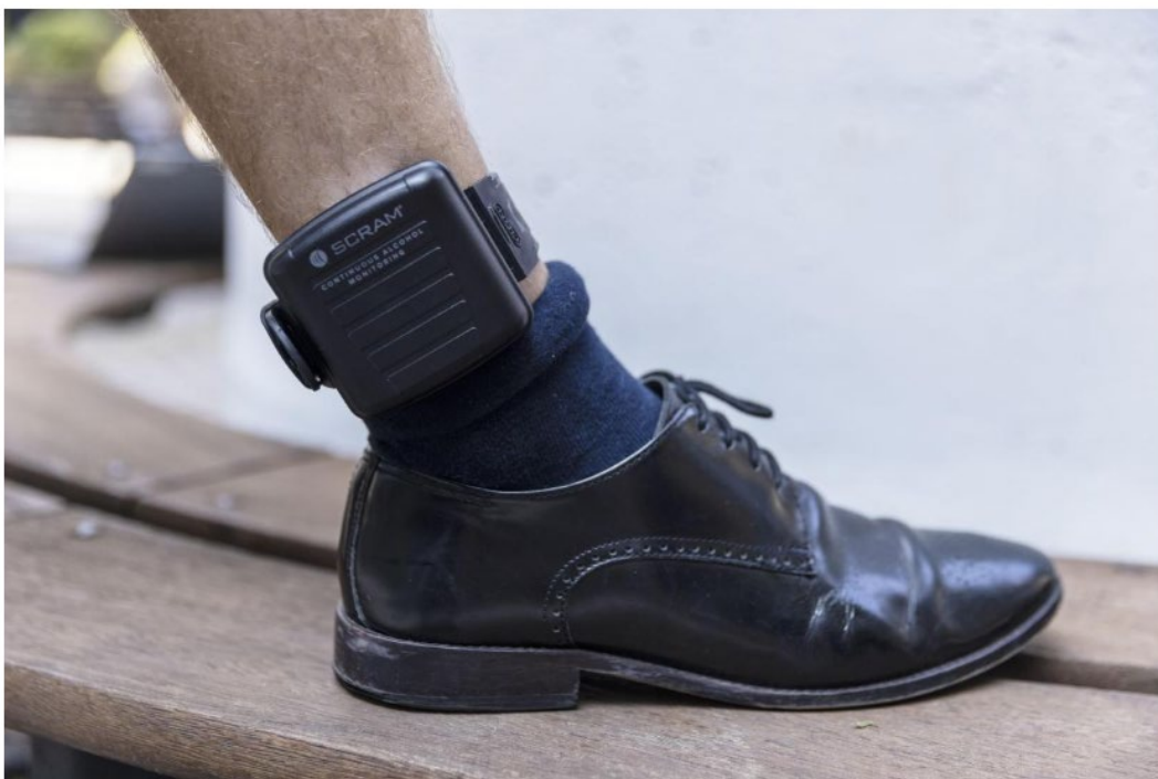
The device can detect alcohol in the body by monitoring sweat TIMES PHOTOGRAPHER JACK HILL
