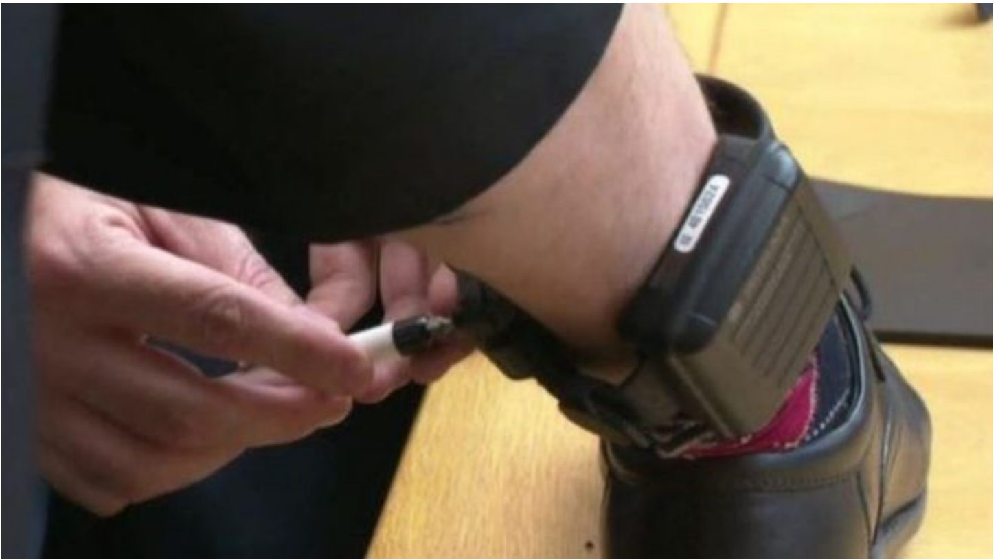
Sobriety tags are ankle bracelets which track alcohol levels in sweat
